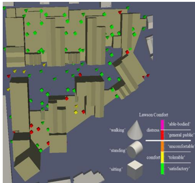
Figure 17.6: Lawson Comfort Criteria Within the Proposed Project Excluding any Landscape Features or Other Mitigation Measures
