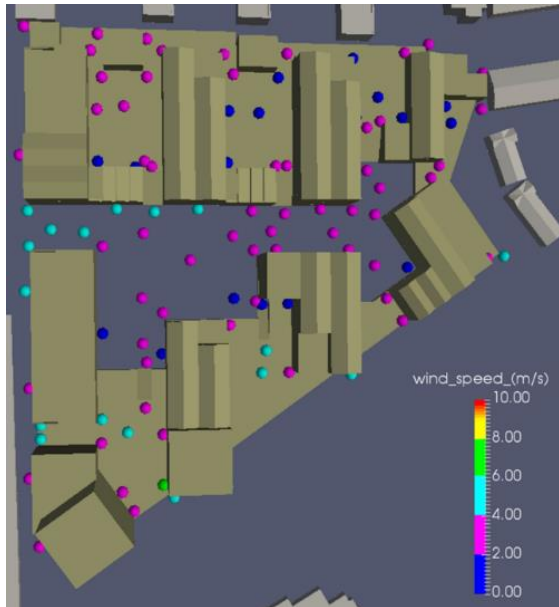
Figure 17.5: Lawson Comfort Wind Speeds Within the Proposed Project Excluding any Landscape Features or other Mitigation Measures
